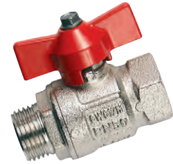
BSP male/female - PTFE seal - vlinderhandel
