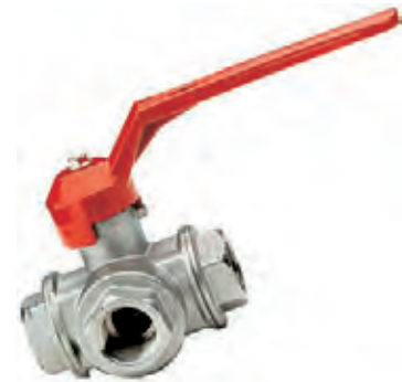
BSP female - L-boring - PTFE seal
