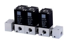
Modular system consisting of direct acting 3/2-way or 2/2-way solenoid valves normally closed, actuated by permanent signal and endplates for common pressure supply (1). Port 2 is in the valve, G 1/4", exhaust through the operator tube, thread G 1/8".
